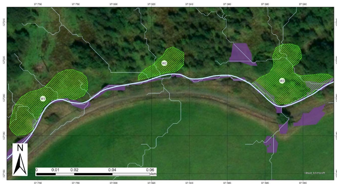
Figure 9 Map of wetland opportunities: Wetland 1 (W1), Wetland 2 (W2), Wetland 3 (W3). Thinner blue lines represent flow paths into Lottice Brook (Thicker line), data collected from SCALGO live. Purple shapes represent depressions in the ground.
